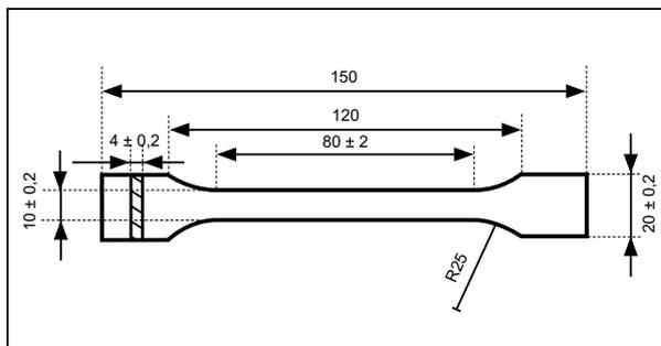
Testspecimen type 1A
