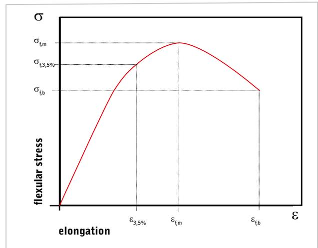
Flexural stress- outer fiber strain
