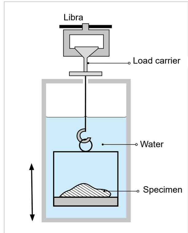
Density measurement, archimedes principle
