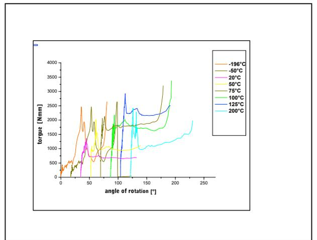
**Example:** Determination of switching torque of a ball valve with ball seals from ZX-324 at extreme temperatures from -196 to + 200 ° C
