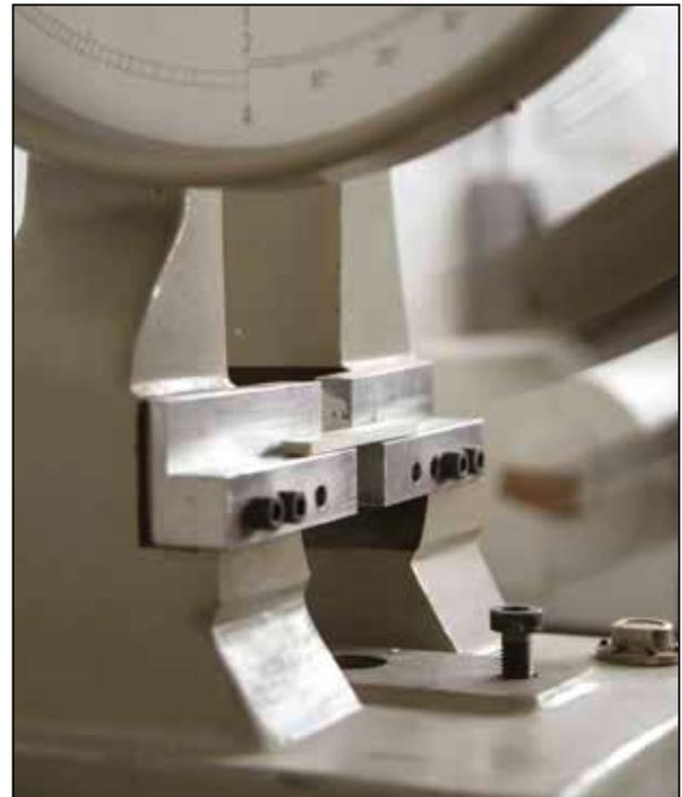
*Impact strength testing device*
