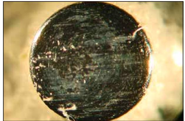
*Covering material after 120 min. 6x magnification, specimen with oscillating wear track.*
