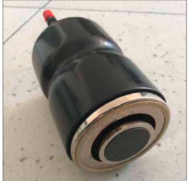
*Surface resistance measuring electrode*
