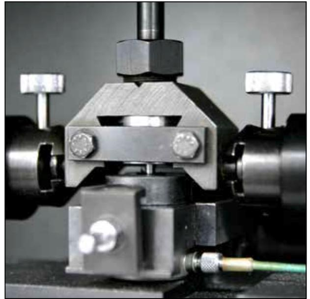
Oscillation block with test specimen
