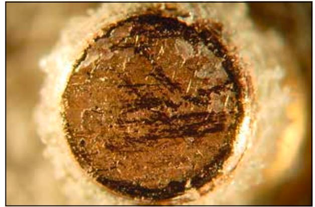
*Covering material and specimens with oscillation-wear track.*
