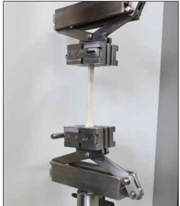
Experimental setup (in this case: tensile creep test)
