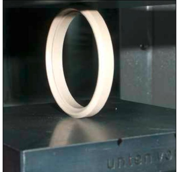
**Example:** Pressure test on sealing rings from ZX-324 (axial and radial). It was determined, in which force a permanent deformation occurs respectively at which force the rings break
