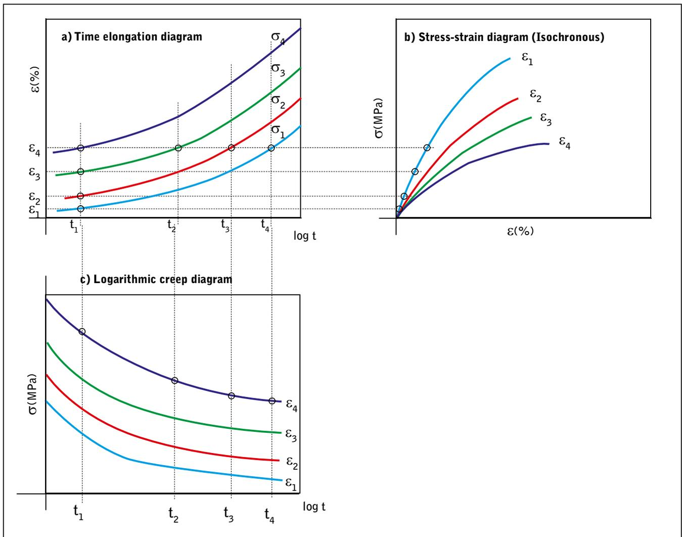
*Deformation and stress at different loading times*
