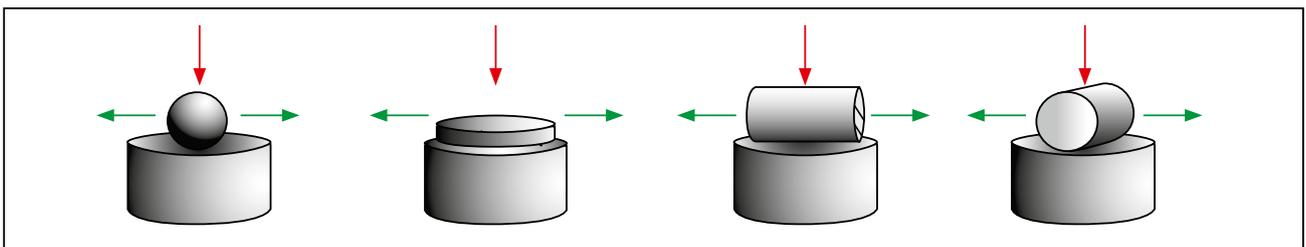
*Contact conditions are point, line, or contact surfaces of the specimens.*
