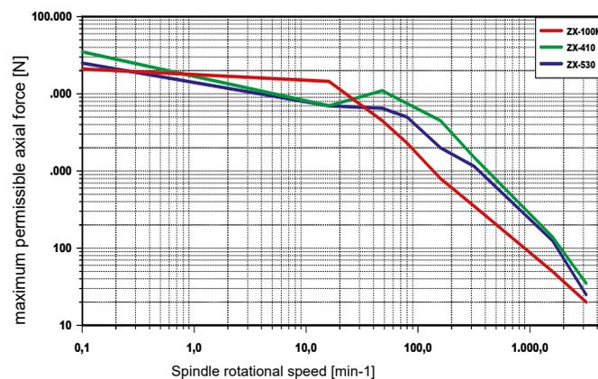
*Axial force in dependence of the spindle rotational speed*
